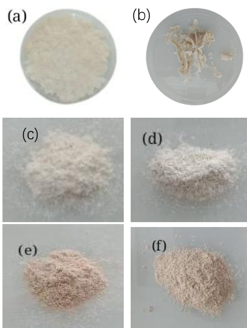
figure 2: Cellulose fiber in wet state (a), Cellulose fiber in dry state (b), Cellulose fibers extracted from U. lactuca using 10% NaOH (c), Cellulose fibers extracted from U. lactuca using 20% NaOH (d), Cellulose fibers extracted from U. lactuca using 30% NaOH (e), Cellulose fibers extracted from U. lactuca using 40% NaOH (f).
